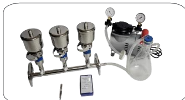
Vacuum Filtration Manifold Complete Kit (Stainless steel Filter holder External Clamp)
