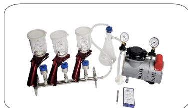
Vacuum Filtration Manifold Complete Kit (Glass Funnel)
